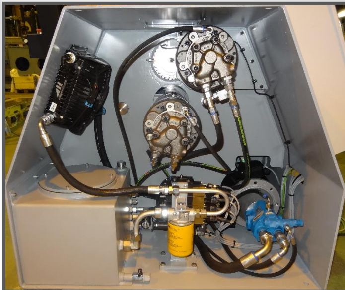
At the back and well protected inside the frame we have placed the hydraulic components, including the oil cooler as an integrated part of the frame. Drive is by separate hydraulic motors and planetary gear boxes for the top and lower shafts.
