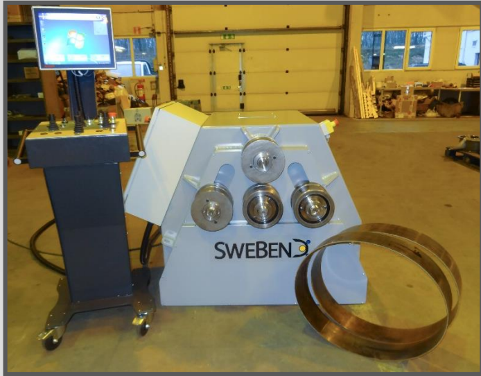
Above: Model SB4B-65 CNC with tooling to allow rolling plates into desired shape, in this case ellipses. Normally this particular product would have been produced in a four roll plate bending machine, but due to cycle time requirement the SB4 model was the better choice.
