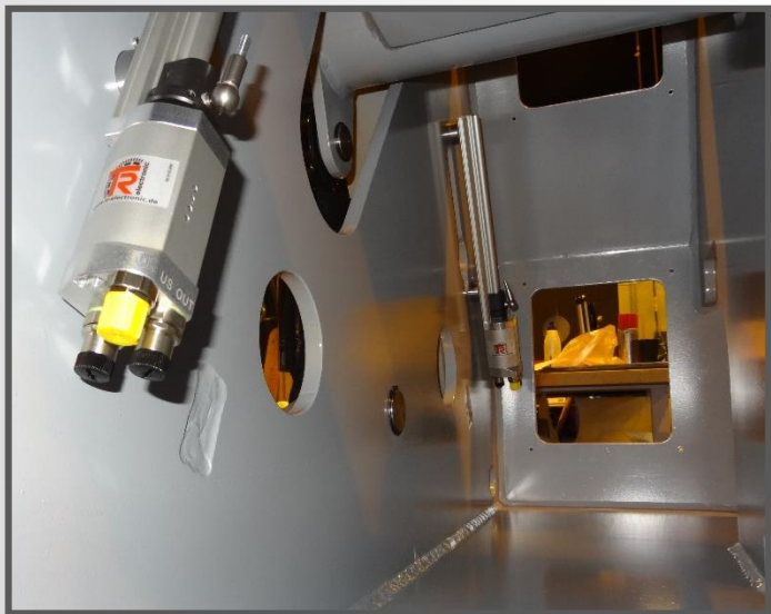
Machine design is made with attention to aspects like how to keep the geometry and machine size compact and yet be able to use the more sophisticated components like linear encoders of absolute type, as shown on the picture above. These encoders are placed inside the frame where they are well protected yet still easily serviced. This is just one detail to explain the way we think and design machines at SweBend .
